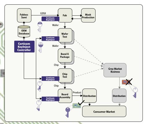
Certicom Security for Silicon Design Protection can be used at every touch point to provide the highest level of security in the chip production process.
