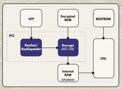
Note: Certicom PCC Core adds 20k gates (2 input NAND equivalent)
